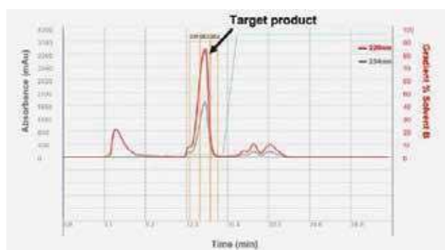
Figure 7. The flash chromatography of the sample by a regular C18 cartridge.
